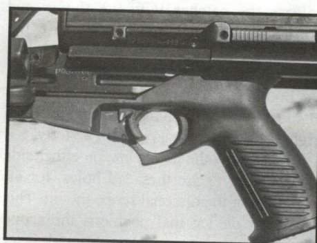
The left side view of the gun shows the charging handle (just under and to the left of the serial number) and the ambidextrous safety/selector.
