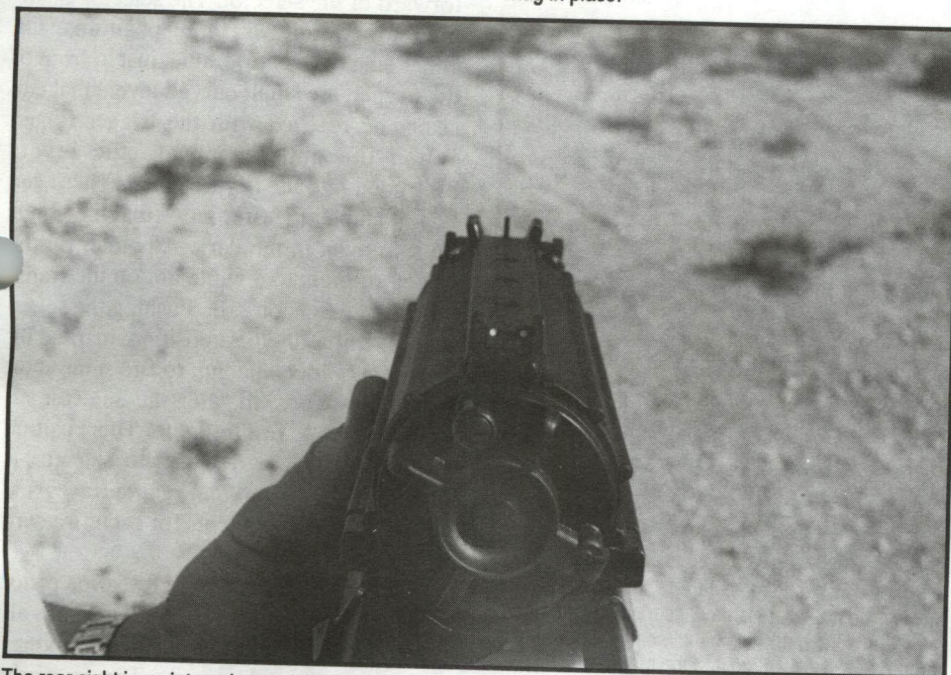
The rear sight is an integral part of the magazine while the front sight is located on the receiver. Also shown in the photo is the clutch release button (in the center) and the fold-out winding handle.
