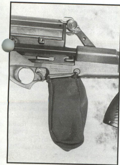
The optional brass catcher is a worthwhile accessory. The bolt release can also be seen just above the selector.
